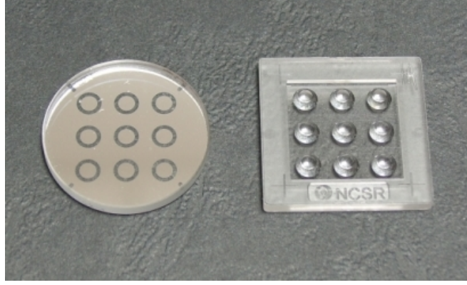
Figure 4.3: Photo of the annular mask and the disposable parabolic biochip
