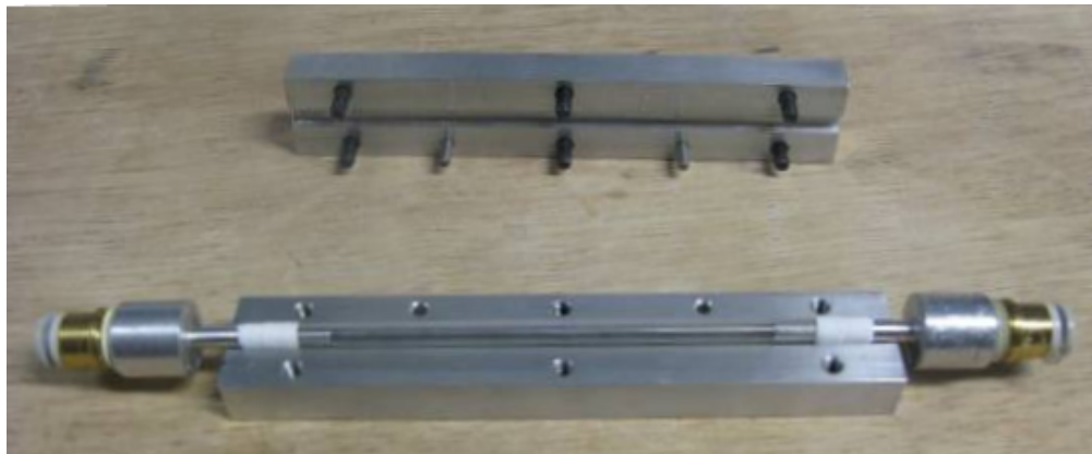
Figure 3.9: Sylgard® filled tube ready for curing.
