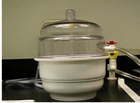
Figure 3.6: Nalgene dessicator attached to vacuum pump
