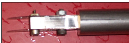
Figure 3.4 (a): Cutting device for ring shaped samples
