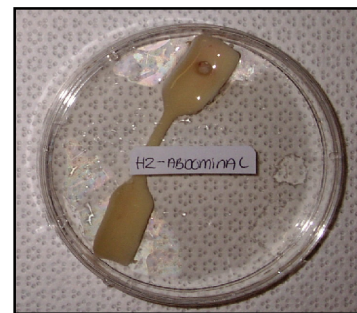
Figure 3.3 (b): Dogbone-shaped sample
