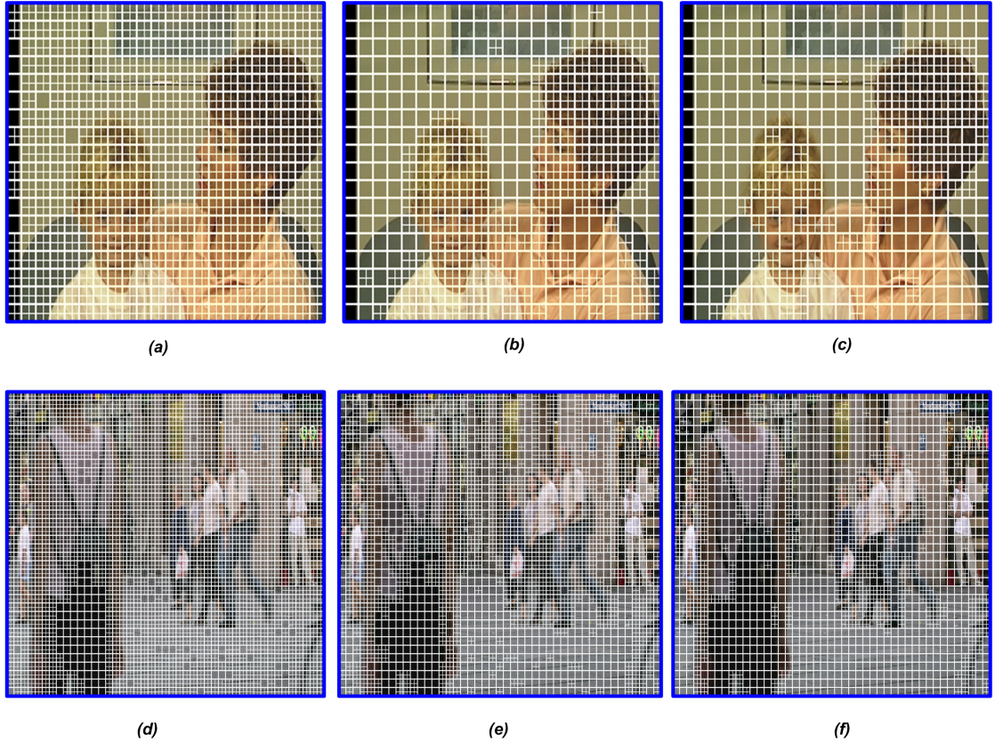
Figure 5.8: VBS partitioned results at various threshold value ( \tau ); (a)(b)(c) are Mother sequence@ 352 \times 288 , (d)(e)(f) are Pedestrian@ 720 \times 576 ; threshold value ( \tau ) are 5, 10, 20 respectively from left side (Note that 4 \times 4 blocks are not displayed intentionally for clear view).
