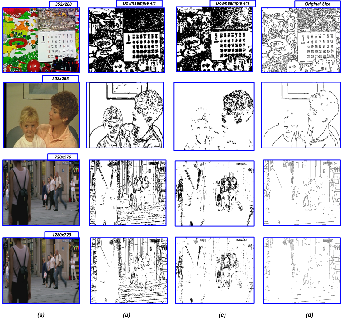
Figure 5.3: Motion edge and edge detection results (a) original image (all images are the 46 th frame ); (b) 4:1 down sampled binary edge images; (c) 4:1 down sampled binary motion edge images; (d) binary edge images obtained by Canny edge detection, where double threshold values are [100, 180]
