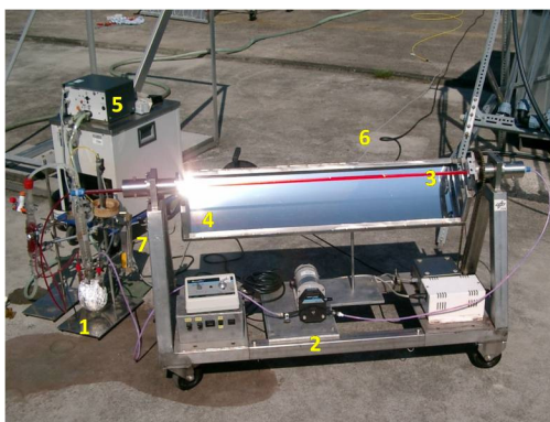
Figure 54: Laboratory scale parabolic trough reactor (1: Collection flask, 2: Pump, 3: Pyrex tube, 4: aluminium mirror, 5: chiller, 6: oxygen supply tube, 7: flow meter).
