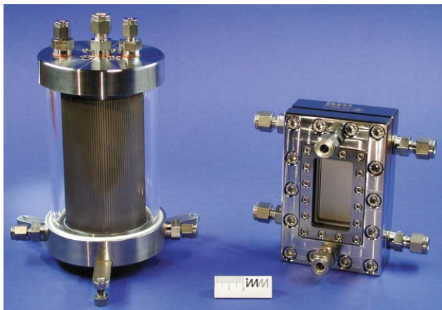
Fig. 2 Cylindrical falling film micro reactor (FFMR-cyl) for 10-fold scale-up and its standard version FFMR (with courtesy of IMM). 29
