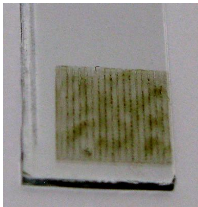
Figure 3.11: Digital image of inkjet printed ITO electrode with vertically aligned SWCNT forests. Square size is 1 \times 1 \text{ cm}^2 , 40 \text{ }\mu\text{m} resolution with an angle of 9.1^\circ .
