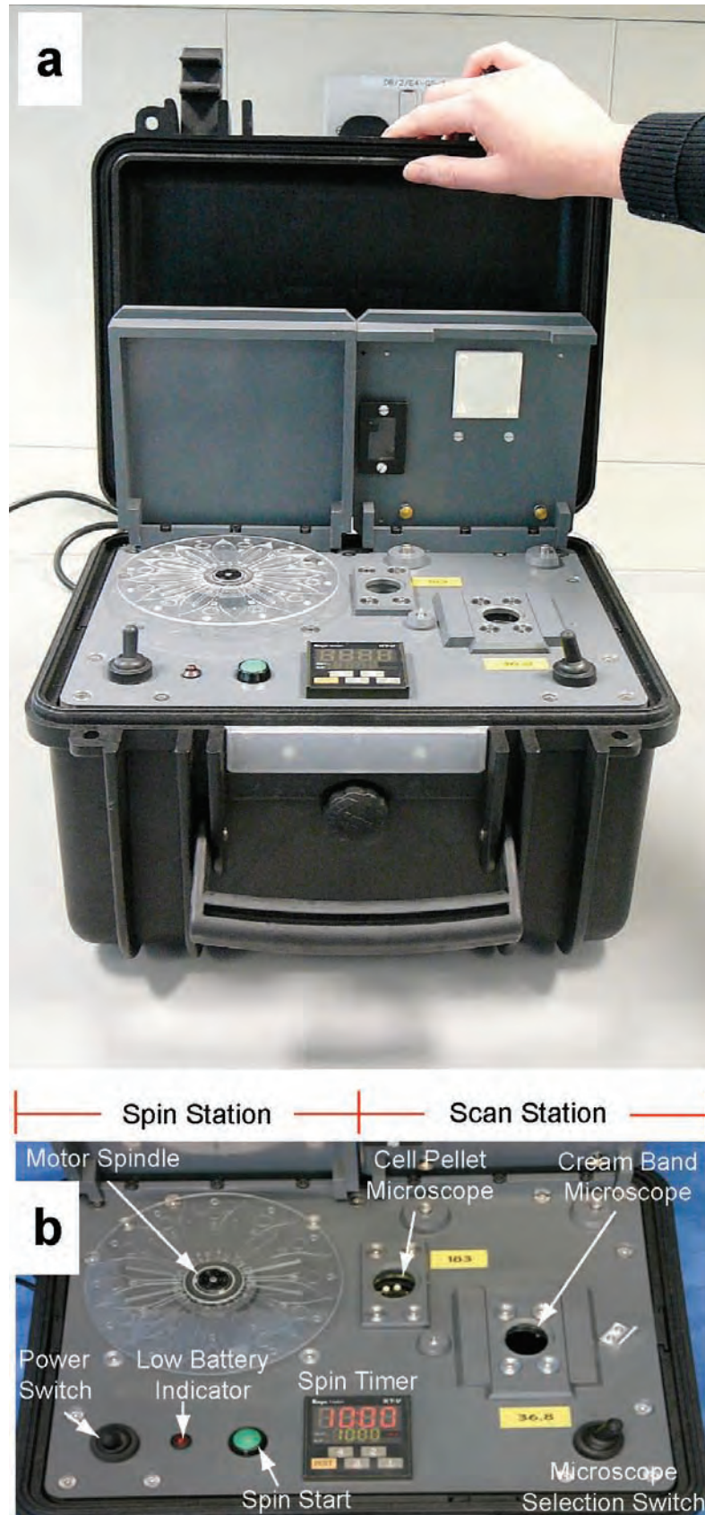
Figure 3.13 (a) Point-of-Cow sedimentation cytometer reader system. (b) The reader consists of a spin and a scan stations to facilitate and automate the cell pellet and band cream measurements.
