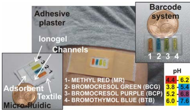
Figure 3: Digital images of the barcode (up right side), the microfluidic platform (down left side) and the incorporation of the platform into a commercially available adhesive plaster (centre); pH dye names and active pH range.
