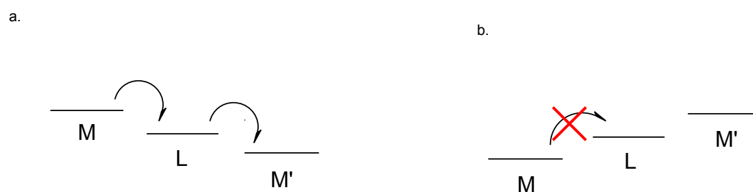
Figure 1.32: Schematic representation of a system in which M and M' are electrochemically different metal centres and L is a bridging ligand allowing electronic communication. Theoretical electron transfer upon oxidation of M is shown where appropriate where M is (a) higher in oxidation potential than M' and (b) lower in oxidation potential than M'
