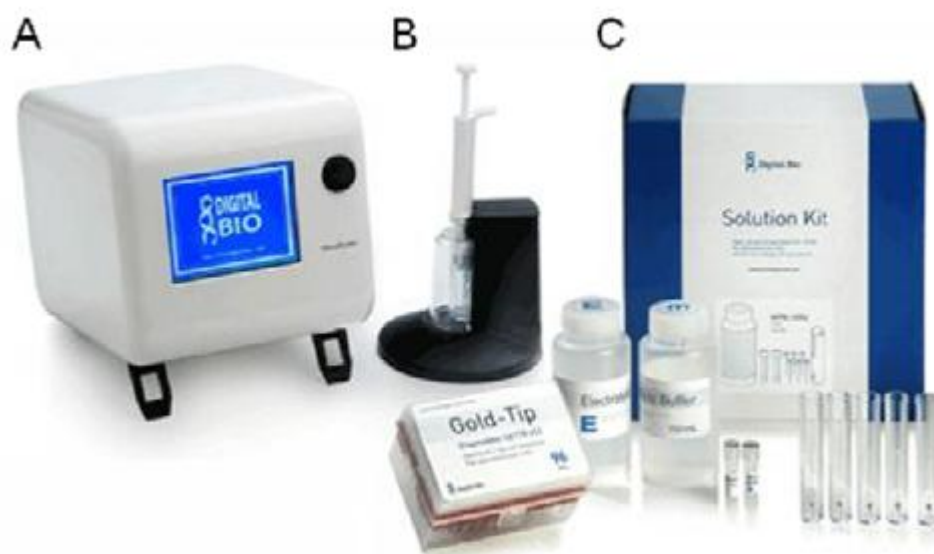
Figure 2.9: The microporator. (A) The microporation unit that generates the electrical parameters necessary for the transfection of DNA and siRNA into cells; (B) The microporation unit consisting of the microporation tube (containing the electroporation buffer) and the microporation pipette used to deliver the electroporation parameters to the cells suspended in the gold-plated pipette tip; (C) The microporation kit containing the necessary microporation solutions, tips and microporation tubes. ( www.microporator.com )
