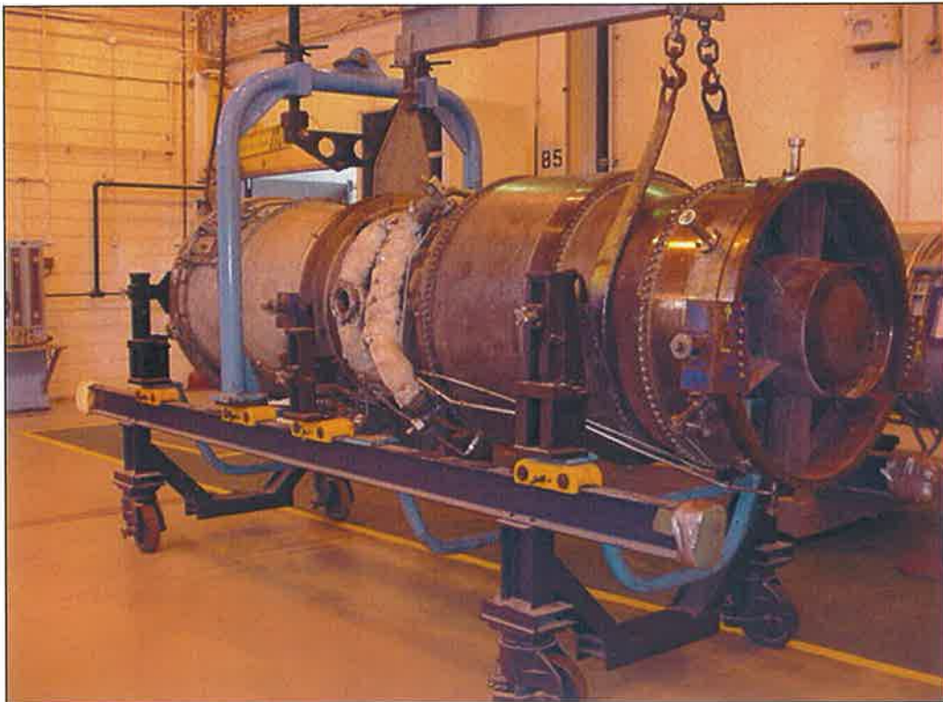
Figure 1, Pratt and Whitney (P&W) FT4-9B Gas Turbine Engine (Saudi Aramco Gas Turbine Repair Shop)
