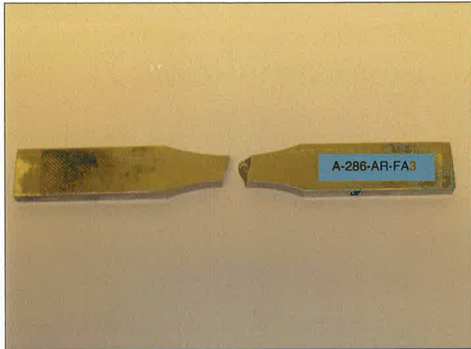
Figure 24, tensile test specimen after failure.
