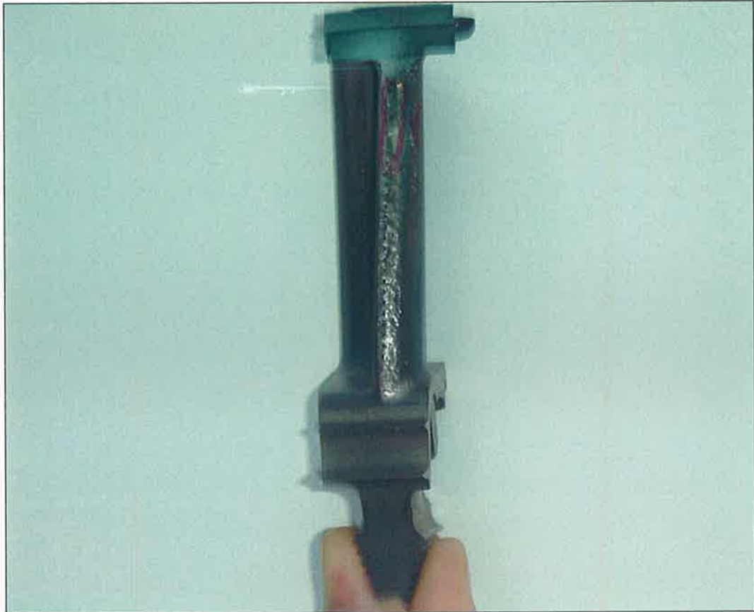
Figure 4, Rolls-Royce RB211-24C heavily eroded 1 st stage turbine rotor blades (Saudi Aramco Gas Turbine Repair Shop)
