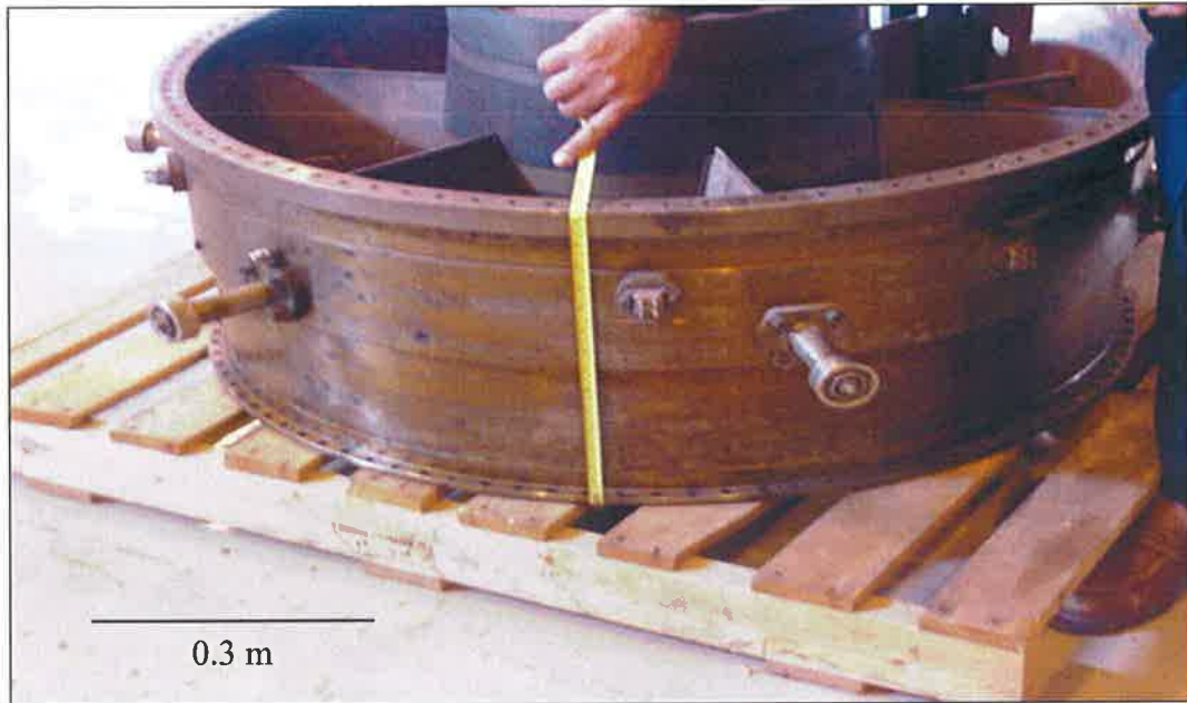
Figure 2, Pratt and Whitney (P&W) FT4-9B Exhaust Transition- Piece (Saudi Aramco Gas Turbine Repair Shop)
