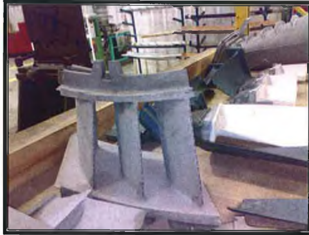
Figure 1.5 application of HVOF coating in Gas turbine component. The coating is AMDRY 9954 and the component is in service in Saudi Aramco.
