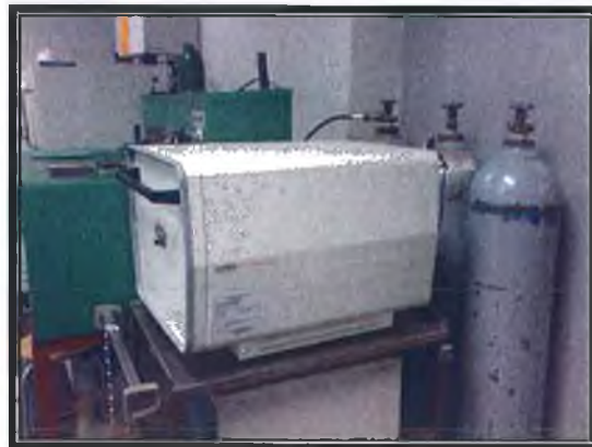
Figure 3.5 Lindberg heat treatment furnace Model 51662
