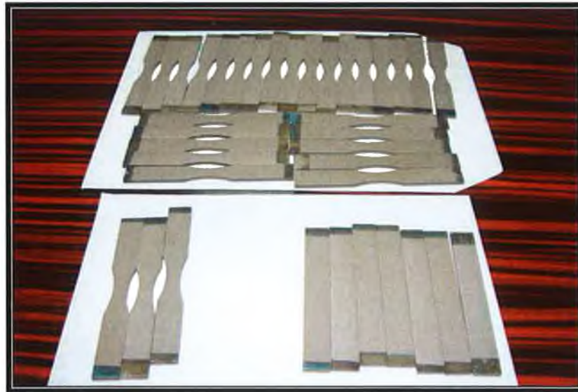
Figure 3.9 Specimens after Coating for three point bending, tensile, and fatigue tests.
