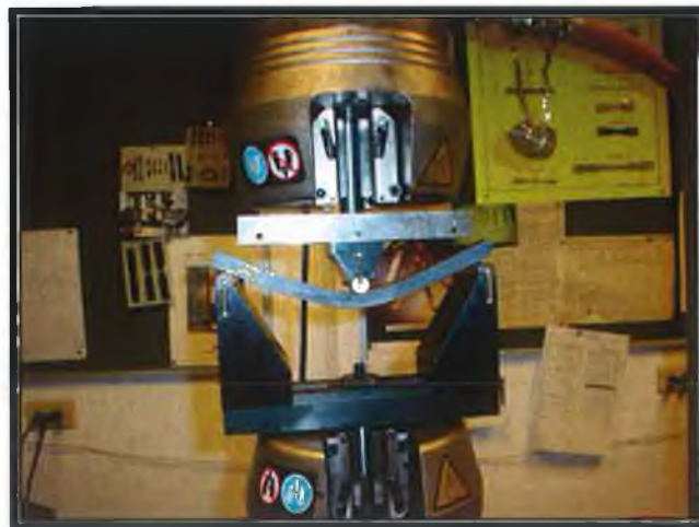
Figure 3.11 – A photograph of three-point bending test set up.
