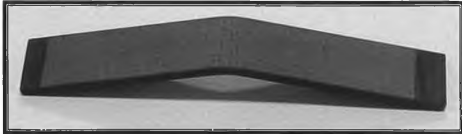
Figure 3.12 – A photograph of workpiece after the three-point bending test.
