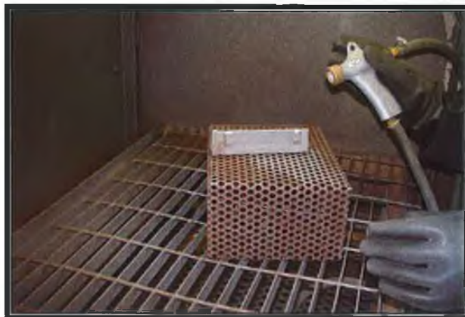
Figure 3.4 Photograph of grit blasting chamber
