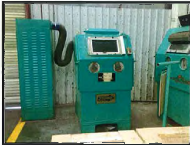
Figure 3.3 Zero Pulsar grit blasting machine
