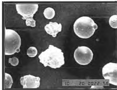
Figure 3.6 – SEM micrographs of AMDRY 9954 powders used in HVOF spraying.
