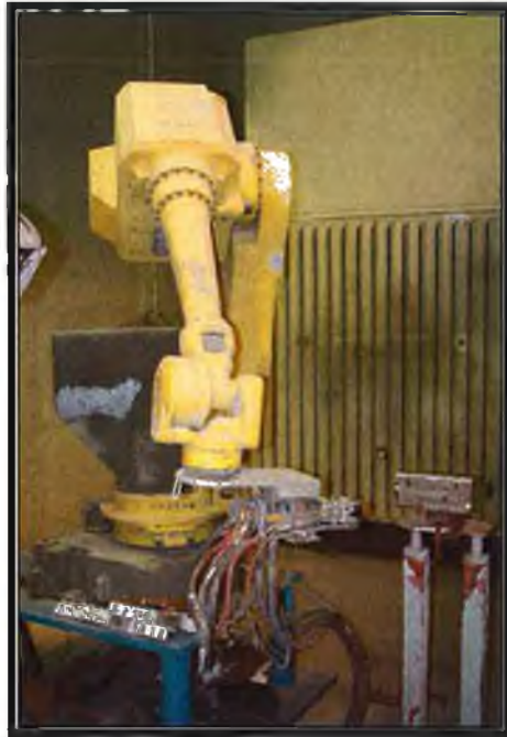
Figure 3.7 Sulzer Metco Hybrid Diamond Jet gun controlled by FANUC Robot M-710i
