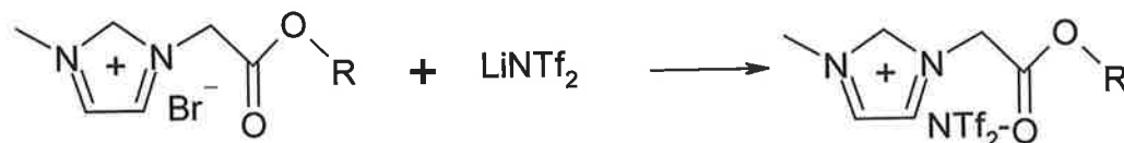
Figure A1.3 Anion Exchange reaction of 3-Methyl-1-(alkyl)imidazolium bromide to form 3-Methyl-1-(alkyl)imidazolium NTf 2 -
