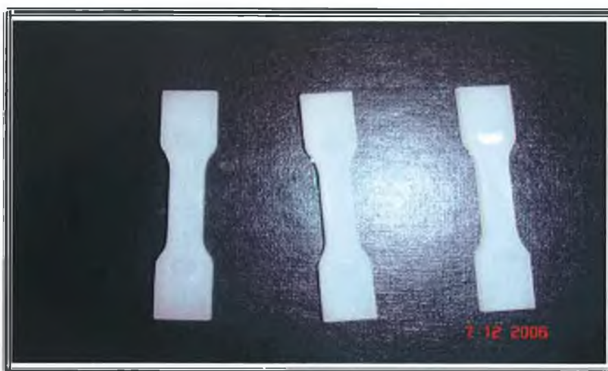
Fig. 3.33: Several of add percentages raw PP with the recycled material PP, (1) first recycle, (2) second recycle and (3) third recycle.
