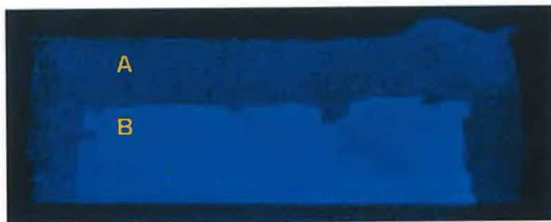
Figure 3.12: Image of fluorescence from labelled antibodies on the chip. Part A: antibodies on the plain region of the substrate (reference) Part B: antibodies on the NP-coated region of the substrate ( \lambda_{res} = 674\text{nm} ).
