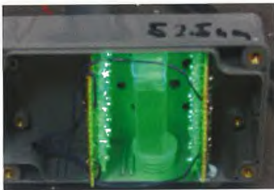
Figure 5.3: LED chamber with 2 x 20 ultra bright LEDs with wavelength 550nm powered by a current source.
