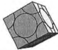
Fig 4.5.1: A section of spheres in CCP packing
