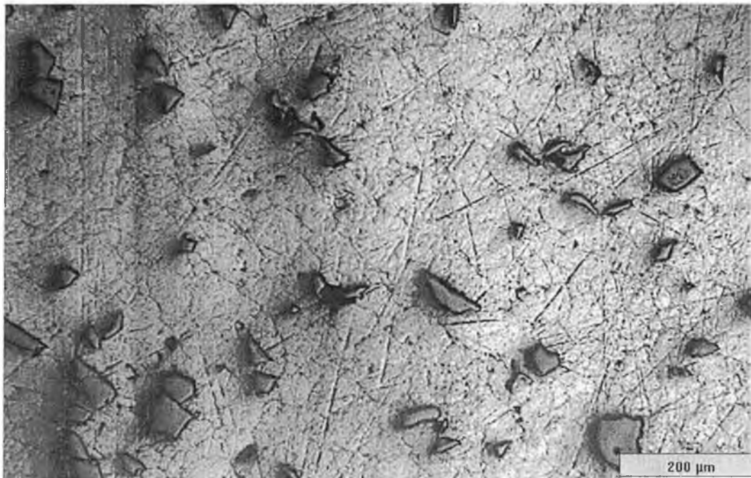
Fig 5.2.5: A sample of 10μm Al + 10% by 23μm vol. SiC p
