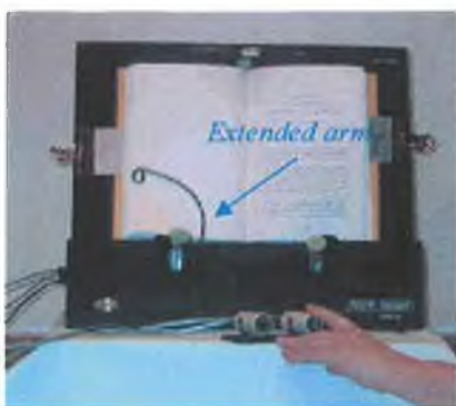
Figure 4.4 Touch Turner illustrating the extended page flipping arm
