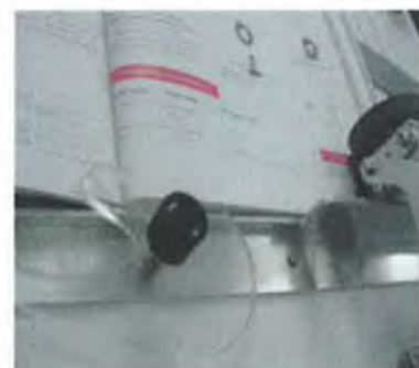
Figure 3.3 Excessive pressure from friction wheel.
