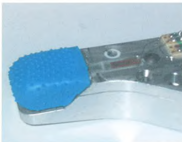
Figure 7.2 Fingertip and Strain Gauge set-up
