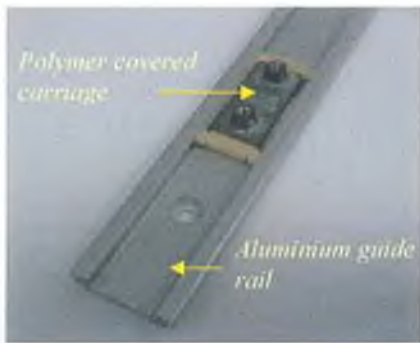
Figure 4.24 Lightweight guide-rail and carriage
