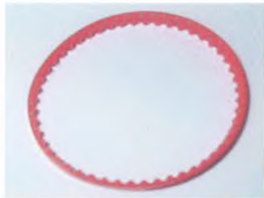
Figure 7.4 Flexible secondary finger drive belt
