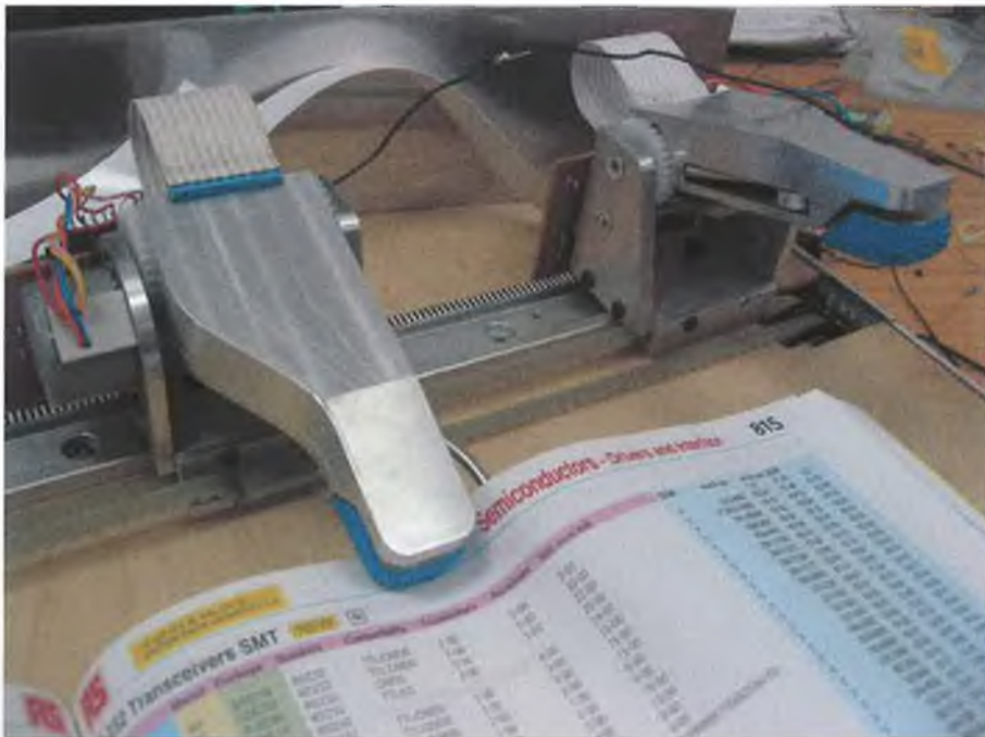
Figure 7.18 Outside finger lifts before inside finger, to allow page to move
