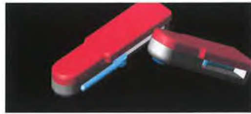
F. Outside finger lifts before inside finger, to allow page to move
