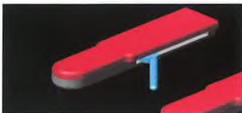
E. Notice motion of secondary finger (centre of rotation offset to allow clearance for page.)
