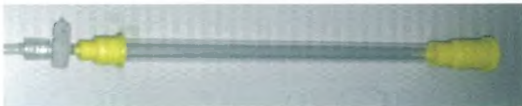
Figure 5.14: The Econo-Column (ID =1cm and length =20cm)
