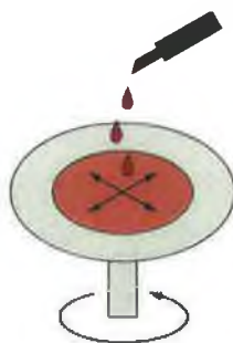
Figure 2.5: Schematic of spin-coating.
