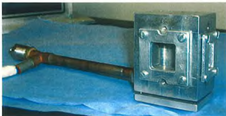
Figure 2.17: Flow cell ( 5 \times 3 \times 1.5 cm) with gas heater attached on the left side for sample characterisations (concentration and temperature runs).
