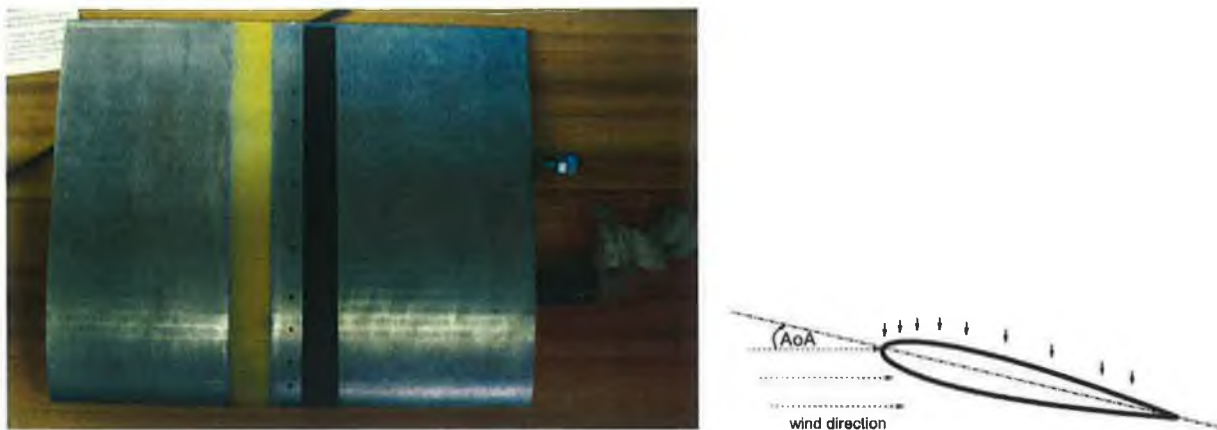
Figure 6.1: Left: NACA 0012 airfoil before the wind tunnel test. The black dots in the middle are the inlets to the pressure taps and on the right-hand side of the image is the plastic tubing used for the connection of manometers. To the left of the pressure taps is the yellow strip of the PSP&TSP paint (on the right of this is a black strip of paint from another experiment). Right: Cross section of NACA 0012 airfoil at a positive angle of attack. Arrows show the approximate position of the pressure taps shown in the photograph on the left.
