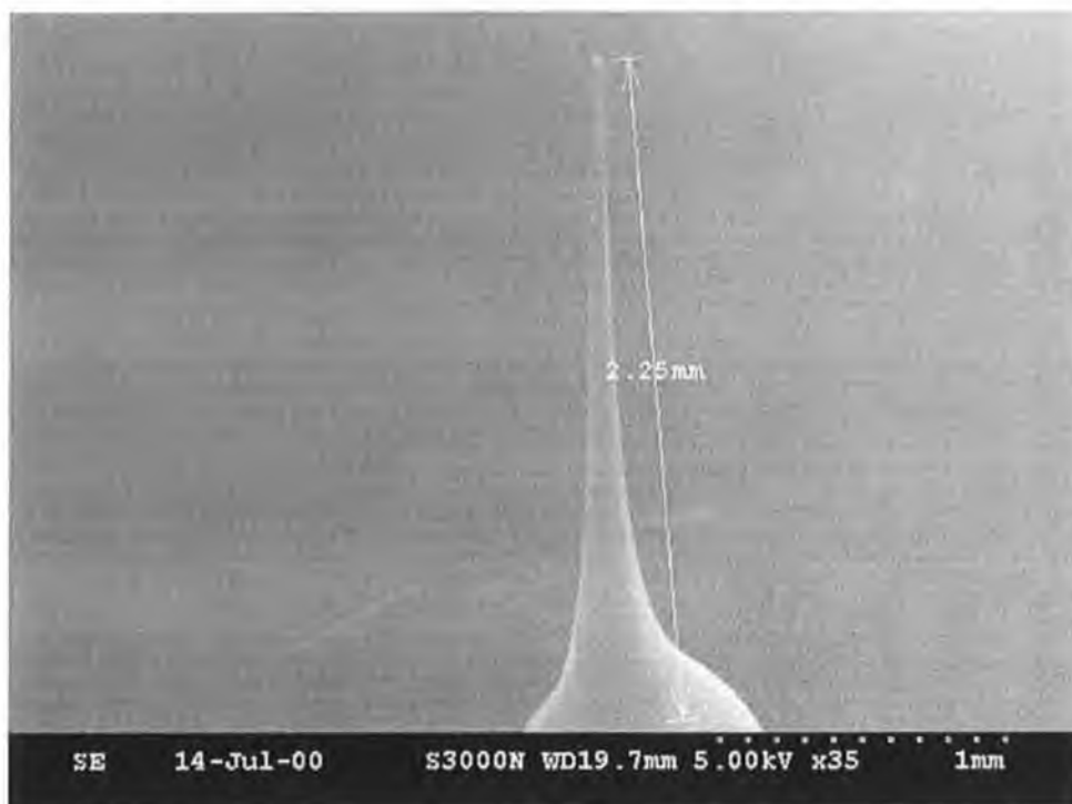
Figure 14. Scanning electron micrograph of a nanoelectrode which has been fabricated using the P-2000 Micropipette Puller from Sutter Instruments. The scale, magnification and accelerating voltage are displayed on the image.
