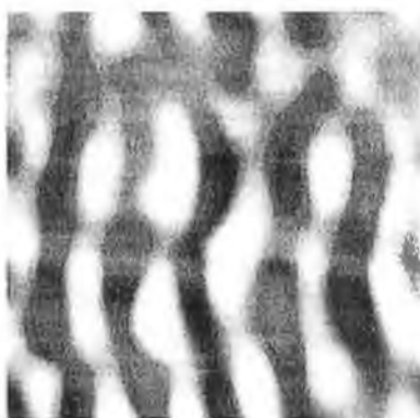
Figure 30. AFM image (3.0 nm x 3.0 nm) of a self assembled monolayer of AQ-2-COOH on silver. Image was FT-filtered to remove noise.
