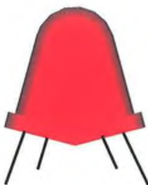
Figure 5-3: Schematic of LEDs fused together at 30° (to the base of the LED).
