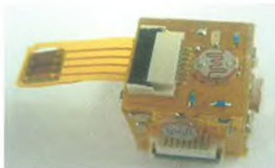
Figure 6-3: Photograph of 10 mm 3 sensor node designed by the Tyndall Institute [7].
