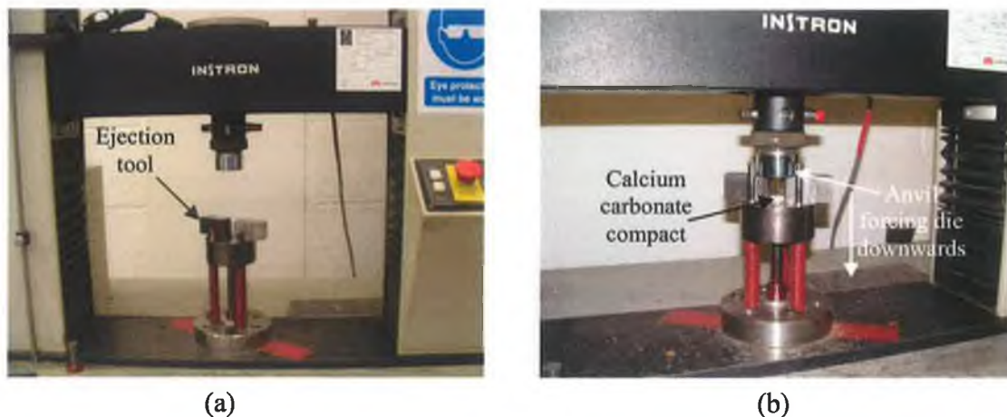
Figure 3.5. Ejection set up steps; (a) positions of the two ejection tool on top of the die body, (b) load applied to eject the compact.
