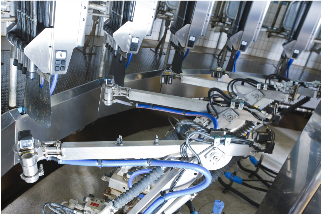
Figure 1.5: DeLaval AMR system showing four robots and no cows.
