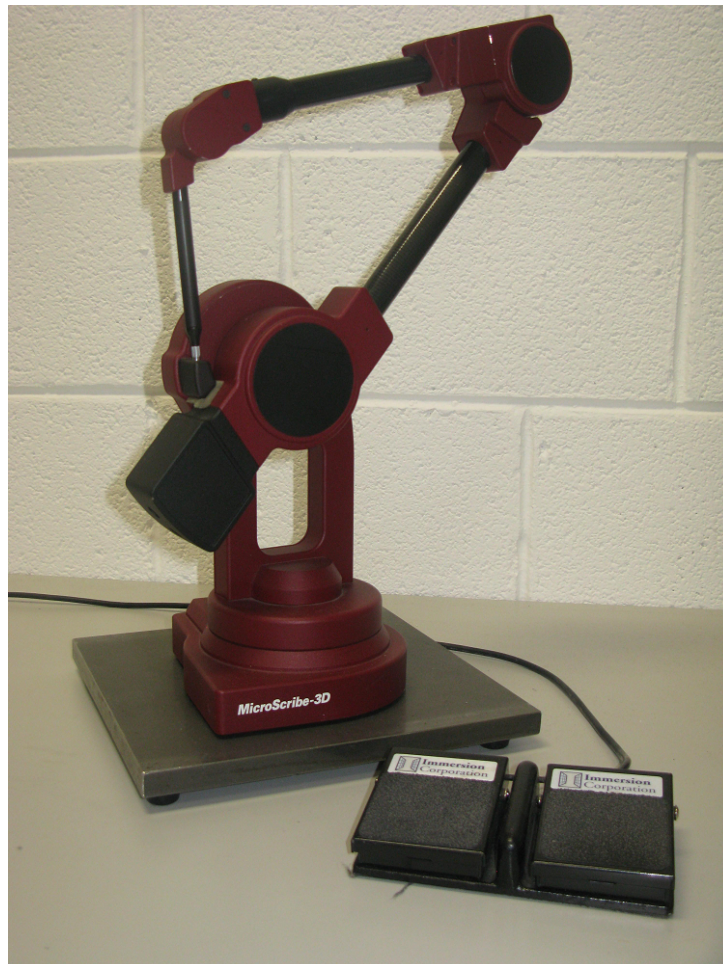
Figure 2.8: Microscribe measurement probe shown mounted to a steel plate with footswitch.
