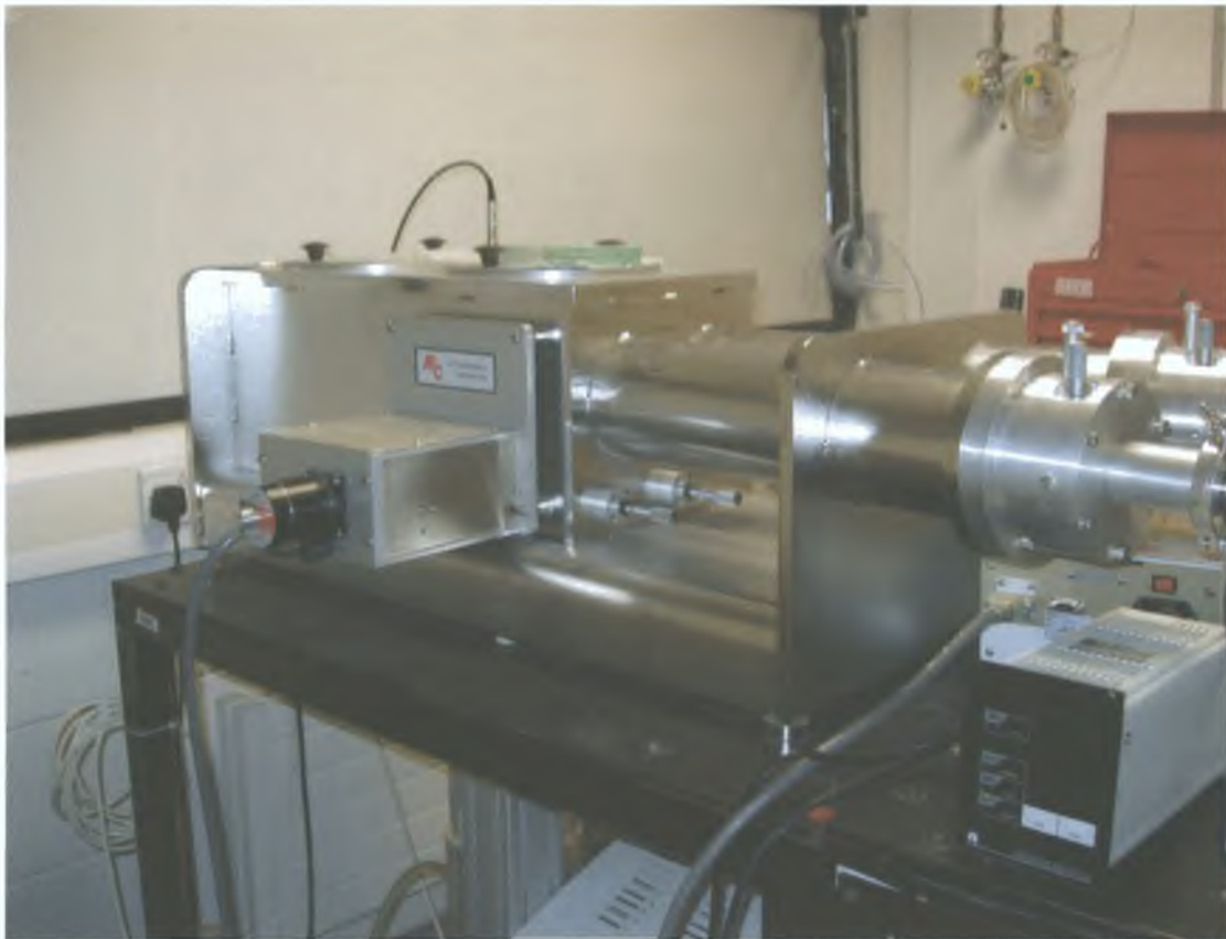
Figure 3-8 The Acton Research Corporation 1 meter normal incidence spectrometer
