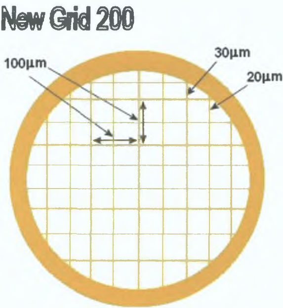
Figure 3-23 Representation of the new 200 mesh grid used to support the aluminium thin films with details of both bar thicknesses and the hole clearly shown
