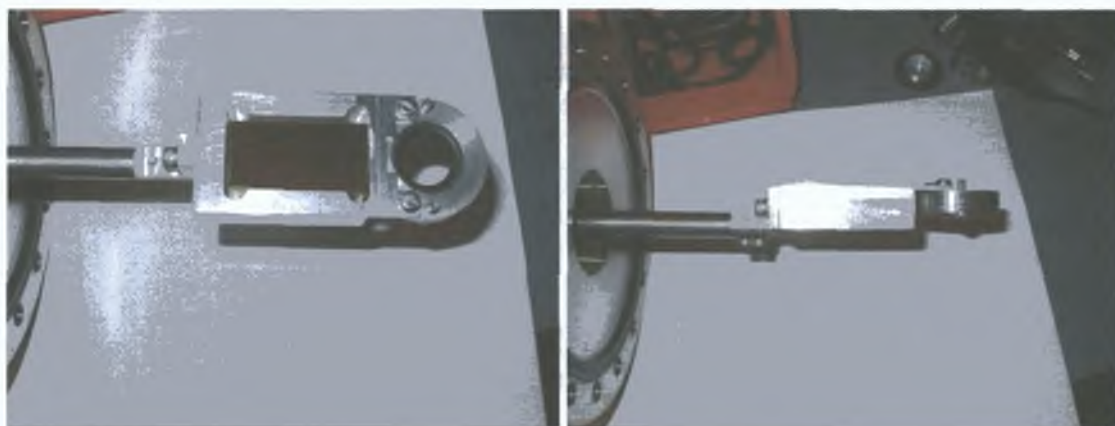
Figure 3-15 Pictures of the sample holder used inside the cross with the gold mirror in place for use in the reflection experiments.
