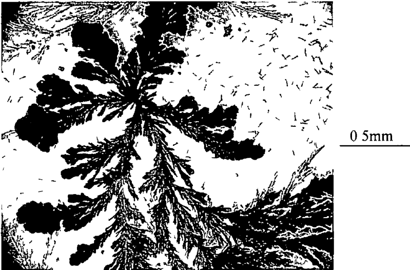
Fig 3.26 Optical micrograph of CuCl thin film on glass two days after evaporation (magnification \times 50 )
