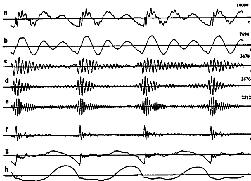
Fig 3 I Inverse filtering analysis (a) speech signal, male vowel [e], (b) waveform of formant F1, (c) waveform of formant F2, (d) waveform of formant F3, (e) waveform of formant F4, (f) double differentiated glottal volume velocity, (g) differentiated glottal volume velocity, (h) glottal volume velocity [after Hess, 1983]
