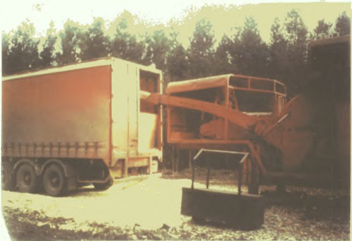
Plate No. 6 : Clean chips being expelled into the back of a lorry through the chute of the Morbark chipper.
