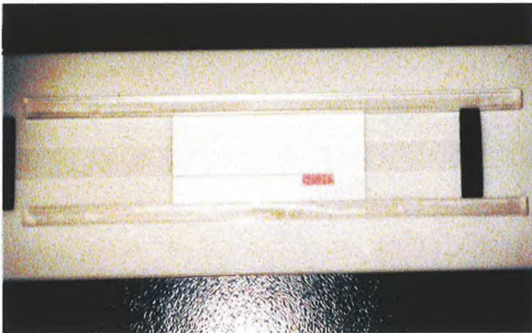
Figure 1.11.8: Photograph displaying the assembly device, which shows a test laminate with the nitrocellulose membrane, gold conjugate and top and bottom pads in position. A section of the bottom pad has been cut away to reveal the pink gold conjugate impregnated strip.
