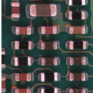
**Figure \$.7:** Image segment (pcb\_3) containing 15 surface mounted components fully within its field of view. (Image supplied courtesy of Agilent Technologies (Ireland), acquired using their *sequential colour* technique at 470, 524 and 660 nm (BGR))
