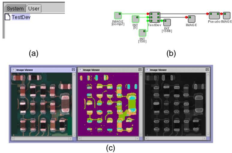
**Figure 4.** Implementation of the `TestDev` class illustrated in Example 3. (a) The associated class file tag in the user area. (b) A sample program illustrating the operation of this block. (c) Sample images (left to right): Input image, K-Means clustered image and the closed structure overlay image.
