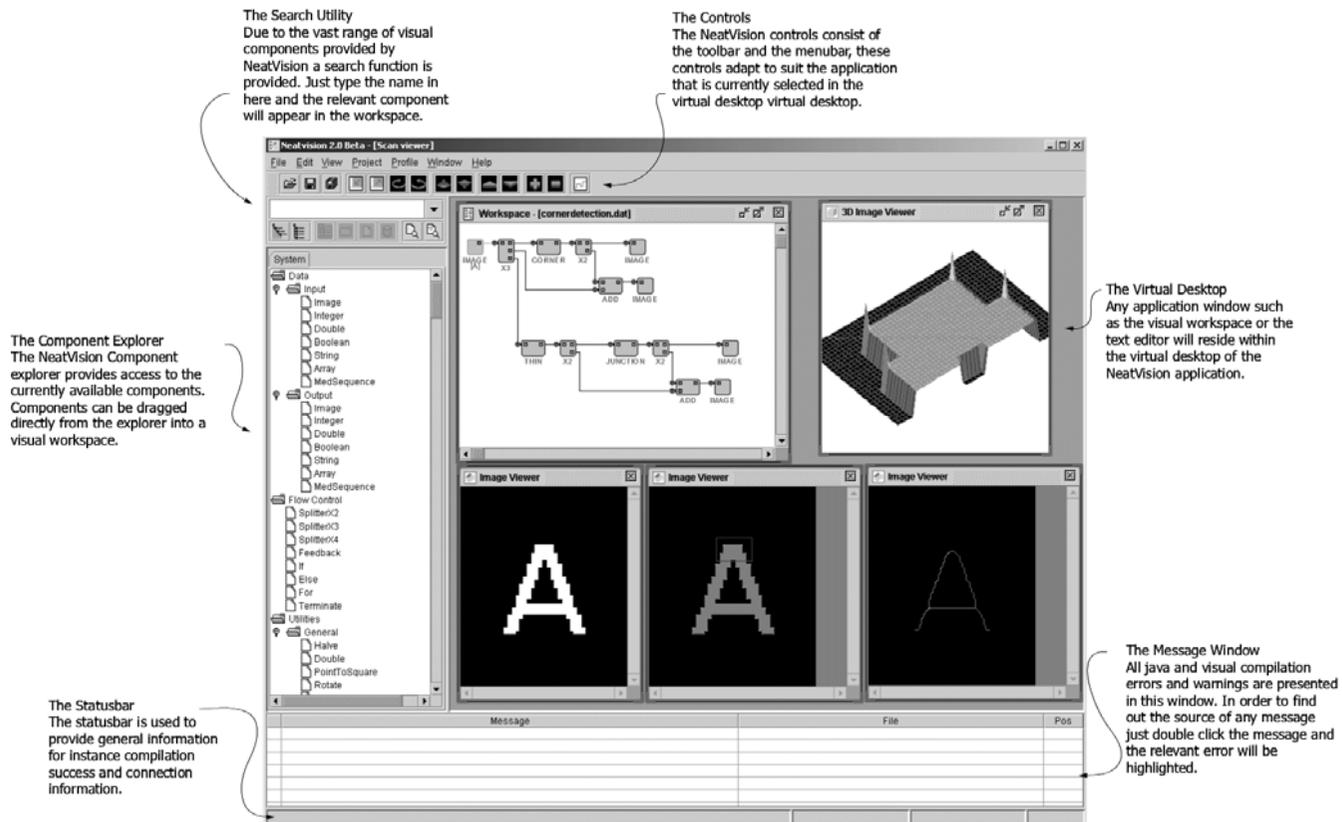
Figure \$.1: Key features of the NeatVision environment.
