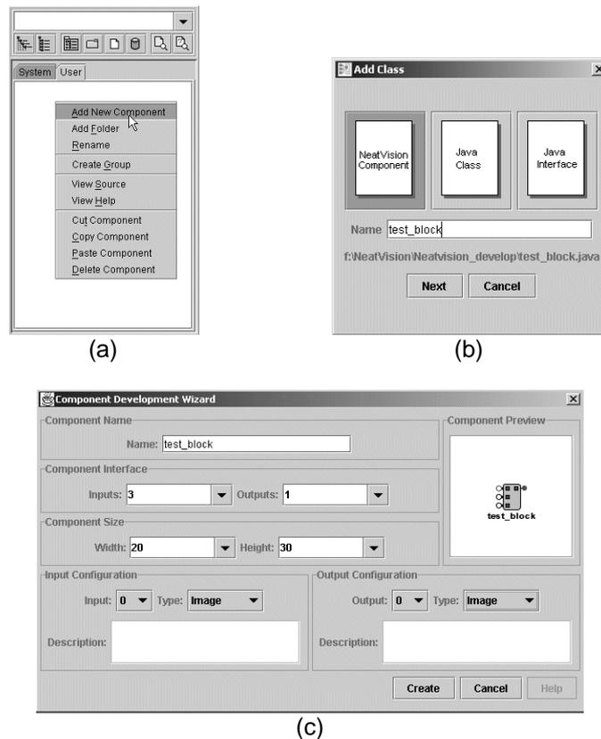
**Figure 3.3:** NeatVision component development wizard. (a) Select *Add New Component* from the popup menu of the *user* area of the component explorer. (b) Select component to be added. (c) Define the component skeleton (i.e. the number and type of inputs and outputs for the associate block). This generates the necessary component wrapping code.
