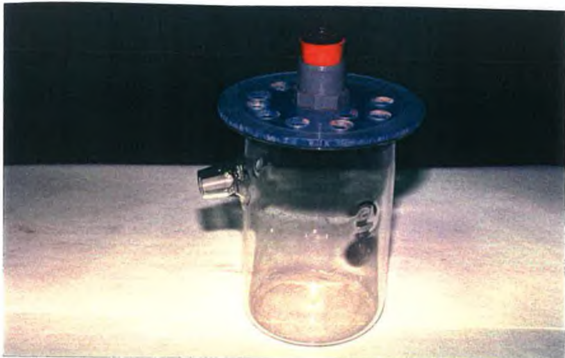
Figure 5.4a The altered fermentation vessel with increased internal effective working area
