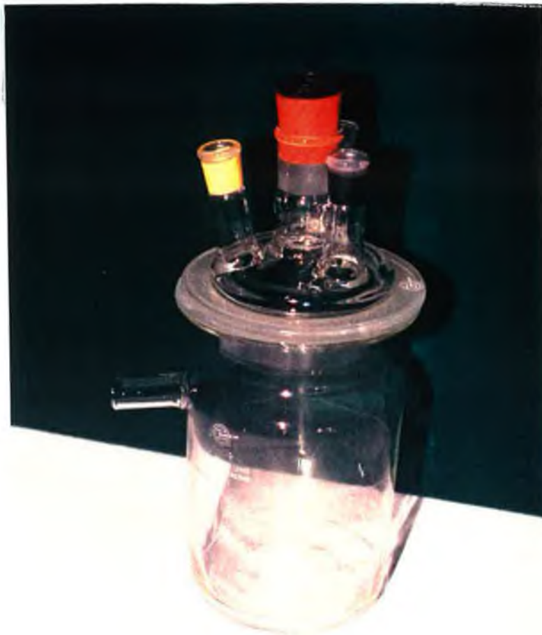
Figure 5.2a Original open waterbath used in the development of the rumen semi-continuous culture
