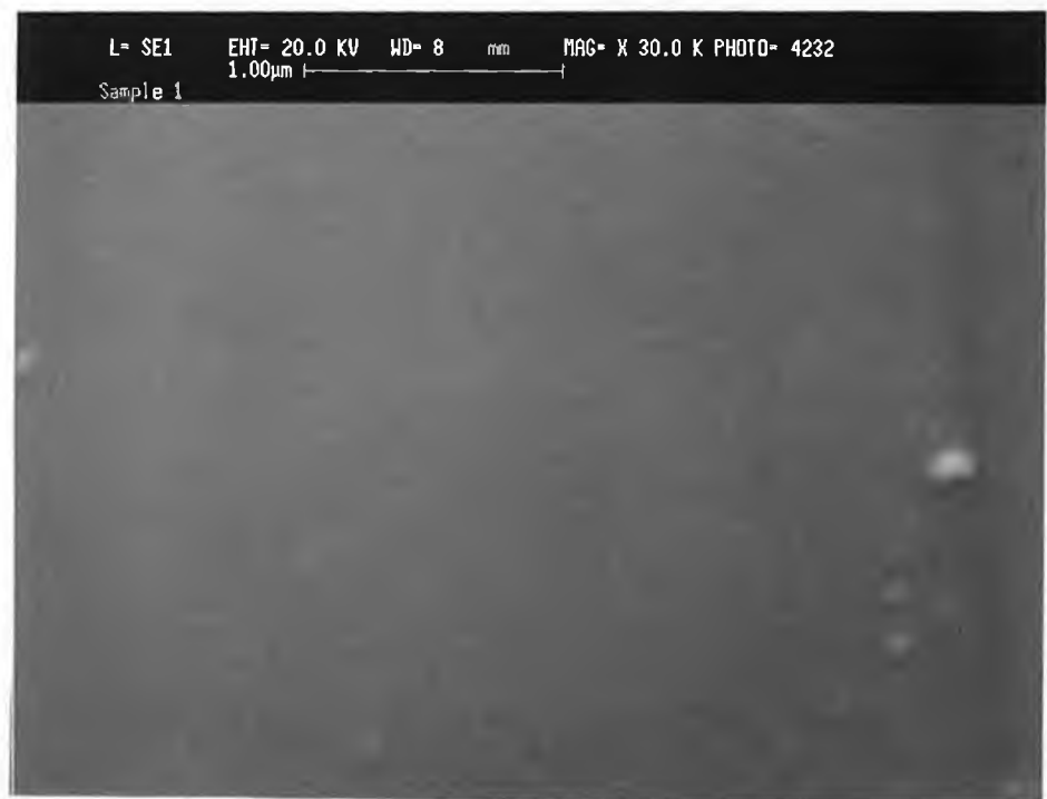
Fig. 4.6(b): SEM micrograph of fig. 4.6 (a) at higher magnification showing an occasional nodule.
