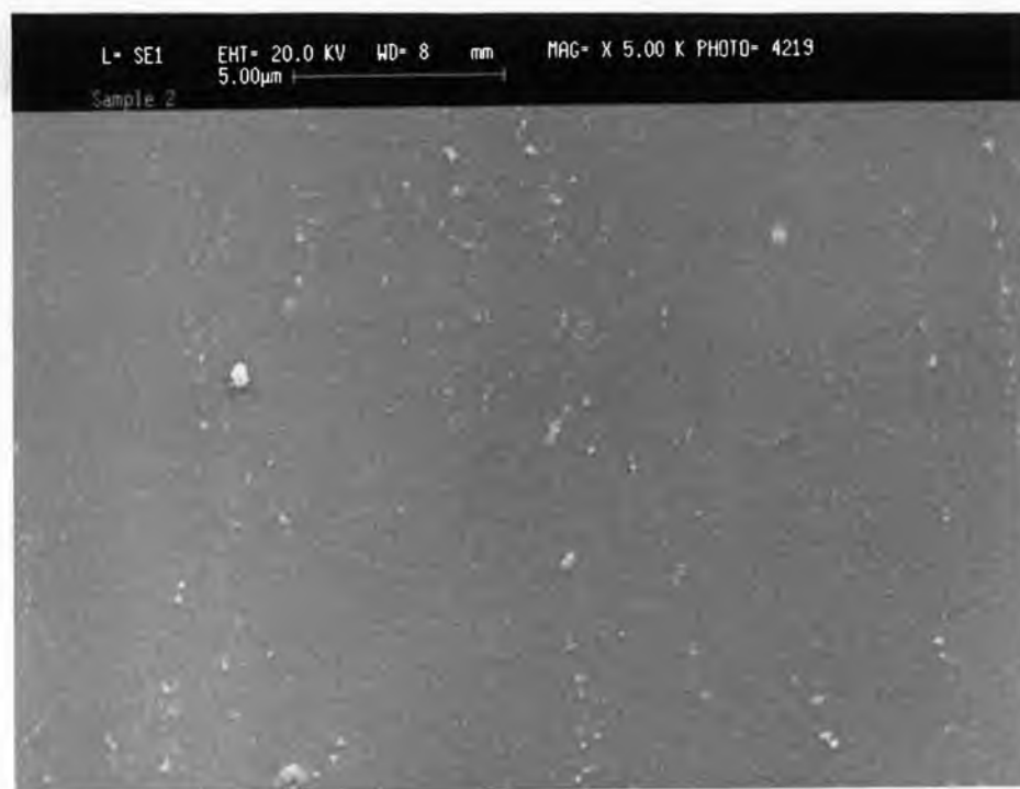
Fig. 4.7(a): SEM micrograph of porous BN thin film on silicon.
