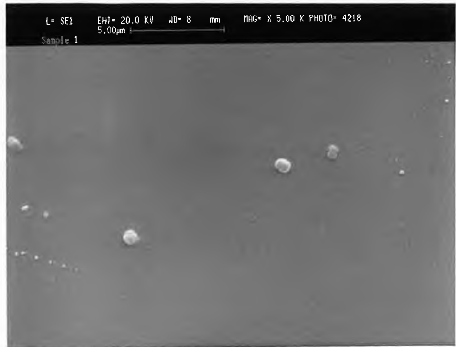
Fig. 4.6(a): SEM micrograph of mixed-phase BN thin film showing smooth surface.
