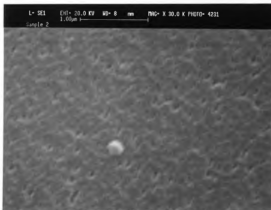
Fig. 4.7(b): SEM micrograph of fig. 4.7 (a) at higher magnification showing microporosity of the film.
