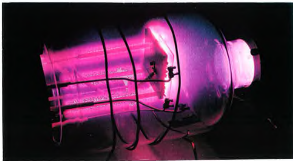
Fig. 4.3: Plasma colour at a rf power of 1) 100 W, 2) 160 W and 3) 400 W.
