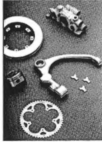
Figure 1.1: (a) Various parts made from aluminium MMCs. (b) Discontinuous silicon carbide/aluminium castings: automotive disk brake rotor, upper control arm, piston, bicycle sprocket, aircraft hydraulic manifold, three engine cylinder inserts. [4]
