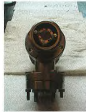
Figure 5.19 Photographs of the analyser assembled and situated in the CF40 T-piece ready to be attached to the chamber.
