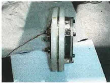
Figure 5.6 Schematic and picture of the overall cathode assembly with external components.
