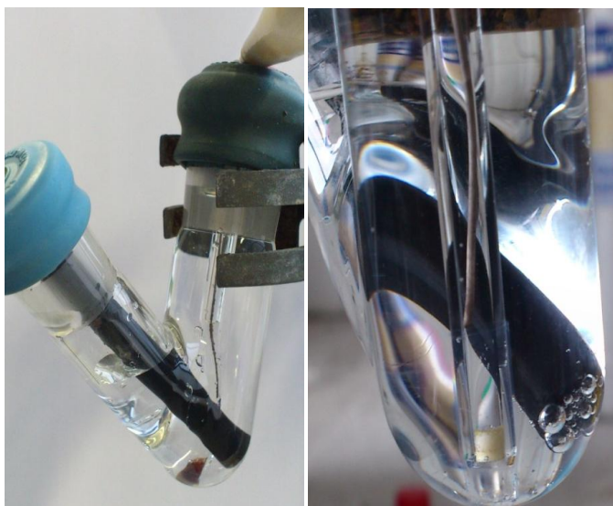
Figure 4.3: Images of experimental set up for the potentiostatic electrolysis of CoPcF_{16} at -1.2\text{ V} vs. Ag/AgCl in 0.1\text{ M NaH}_2\text{PO}_4/\text{H}_3\text{PO}_4 (pH 2). The build up of hydrogen gas bubbles can be clearly seen on the working electrode.
