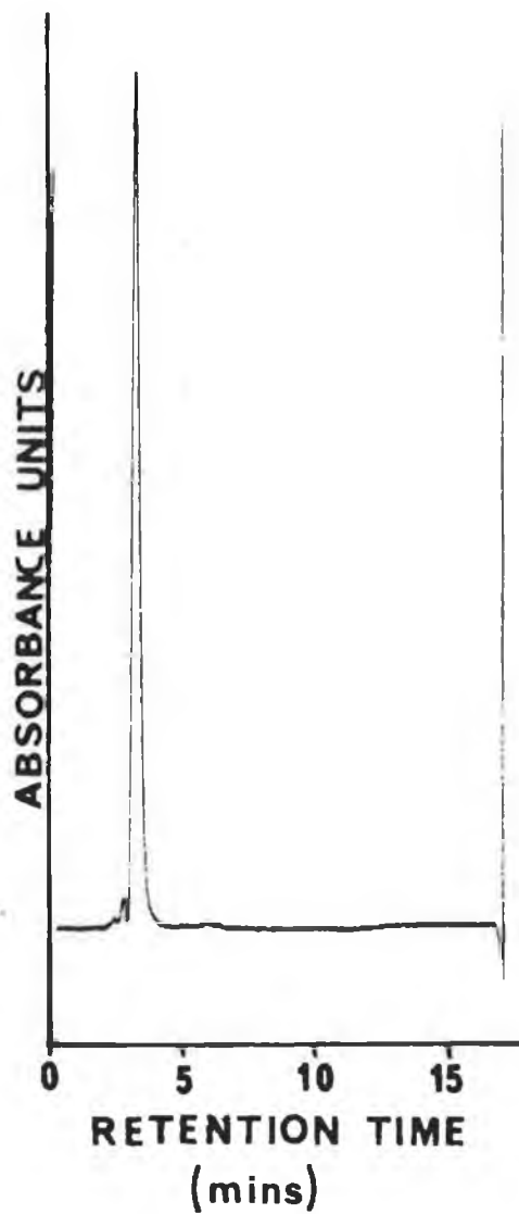
Figure 4.5 The HPLC chromatogram of [\text{Ru}(\text{bpy})_2-(\text{COOHbpy})]^{2+} . The mobile phase used was 80:20, \text{CH}_3\text{CN}:\text{H}_2\text{O} with 0.08 M \text{LiClO}_4 . The HPLC system used is described in Chapter 2, Section 2.2.4.
