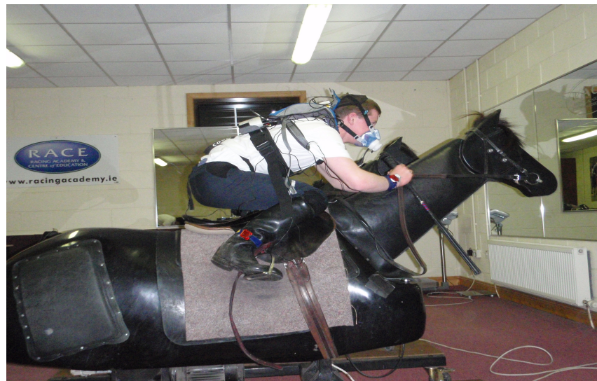
Illustration 3.1: Instrumented Trainee Jockey on Equine Simulator
