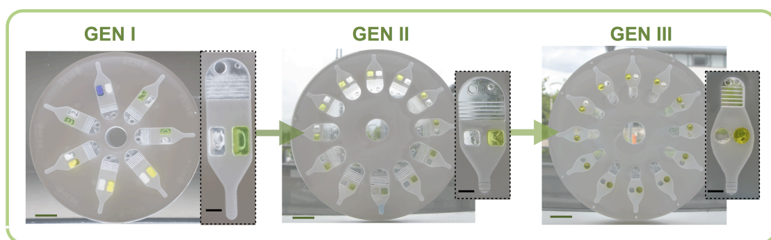
Figure 8.1. Development of the centrifugal microfluidic platform for water pH analysis; the green rulers represent 2 cm and the black rulers represent 0.5 cm.
