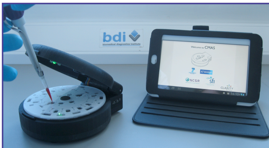
Figure 8.3. Image showing loading of blood sample on the portable CMAS interfacing with an Android tablet. A custom made program was used to control the spinning of the disc and also for wireless real time data extraction.
