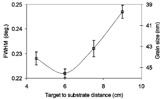
FIG. 3. Variation in FWHM of (111) peak with target to substrate spacing (grain size in the right Y axis).
