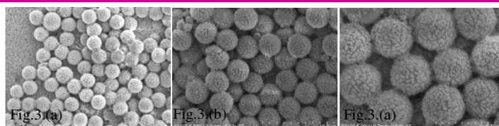
Fig.3.(a-c) SEM images of bimodal structure formed during co-deposition of 200 nm and  $3\mu\text{m}$  PS spheres. During this experiment sonication was used to homogenise the solution. The solution became more homogenised the nano-sized spheres aggregated to the macro-sized spheres Fig.3.(c). However it was found that the  $3\mu\text{m}$  PS spheres settled out of solution very quickly and as a result without constant agitation it would not be possible to pack them successfully.
