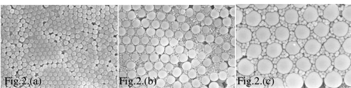
Fig.2.(a-c) SEM images of 200 nm PS spheres and  $1\mu\text{m}$  spheres packed by co-deposition. In this method the two solutions were mixed but no homogenisation of the solution was undertaken. As shown in each of the images (a)-(c) there is a high degree of uniformity amongst the macro-sized PS beads. From this the bimodal structure, most clearly evident in Fig.2.(c) resulted in the nano-sized PS spheres occupying the spaces between the macro-sized spheres.
