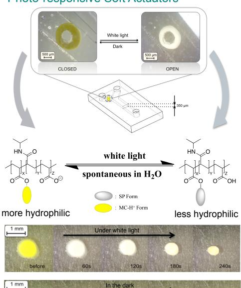
Actuator p(NIPAAm-co-SP-co-AA) micro-structured hydrogels were photo-polymerised through micro-patterned masks. Their photo-induced shrinking and reswelling mechanism was studied under white light irradiation and in the dark. This shrinking and re-swelling cycle can be repeated with great reproducibility.
