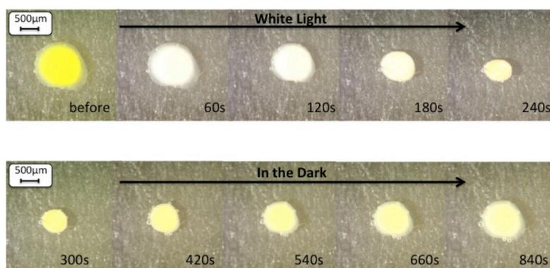
The hydrogels can reach ~49% of the fully hydrated size after 4 min of white light irradiation. After the removal of the white light the hydrogel re-swelled up to ~91% of the fully hydrated size after 11 min in the dark. This shrinking and re-swelling cycle can be repeated with great reproducibility.
