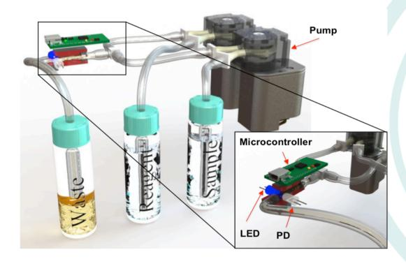
A rendered image of the concept behind the dynamic flow measurement set up. This dynamic measurement will be performed in a microfluidic chip.
