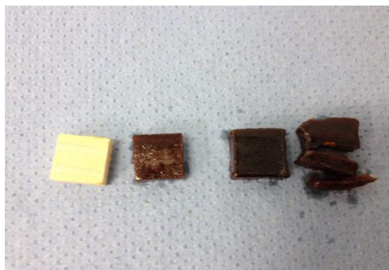
Figure 5.6: Wood expansion states in ILs 190 at 80 °C
