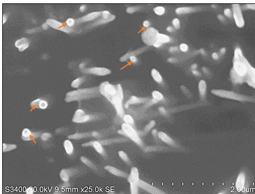
Figure 4.5: SEM analysis of 20 \mu\text{L} drop cast Cu nanotubes placed on carbon tab for analysis (after dissolution of the membrane in dichloromethane, and sonication to remove PC membrane and sputtered gold layer)
