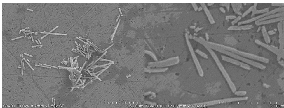
Figure 5.17: SEM images of probe-labelled nanowires confined to electrode surface of a gold electrode functionalised with capture DNA and 1nM target DNA containing a 1 base mismatch via DNA hybridisation following copper shell oxidation at +0.3 V vs. Ag/AgCl in 3 M KCl for ten minutes. The accelerating voltage is 10kV.
