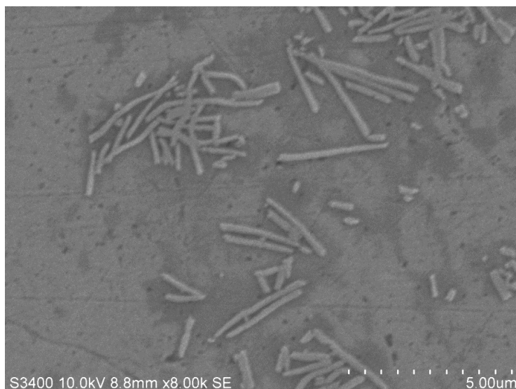
Figure 5.16: SEM image of probe DNA labelled nanowires confined to the surface of a gold electrode functionalised with capture and InM target DNA containing a 1 base mismatch via DNA hybridisation. Accelerating voltage is 10kV.
