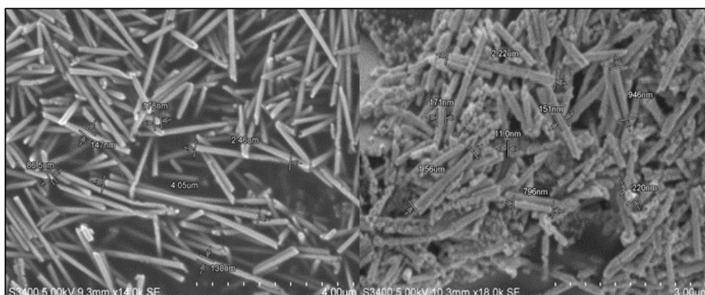
Figure 4.10: SEM images of Cu:Au nanowires from suspension, dropcast onto a carbon tab. (Following dissolution of the membrane in dichloromethane, and sonication to remove PC membrane and sputtered gold layer). The accelerating voltage was 5kV.
