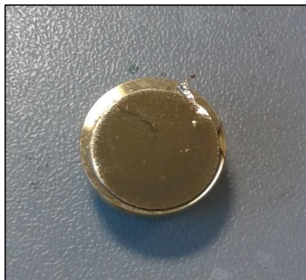
Figure 4.2: Image of membrane following sputter coating with a ~300 nm thick layer of gold before electrodeposition. Membrane was sputtered for 18 mins at a sputtering voltage of 2 kV and a plasma current of 20 mA. (Membrane is mounted on an aluminium stub and adhered with a carbon tab for sputtering).
