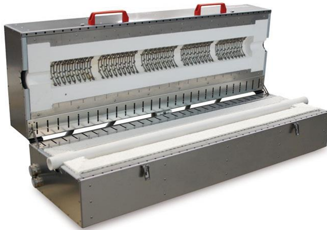
Figure 3.6: Tube furnace used to stress MOS devices.
