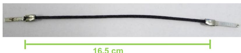
A knitted spandex cylindrical structure with integrated carbon nanotubes (CNT). A variety of sensors were produced with differing core sizes and sensor lengths. Each sensor was tested using the Schober's test as a guideline, focusing on strain percentages surrounding a 6 cm increase.
