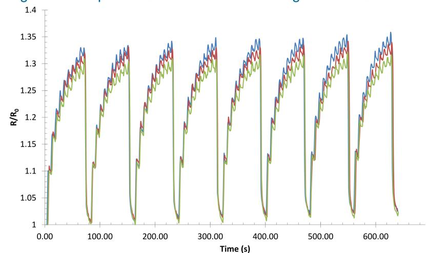
Each sensor was stretched with a linear actuator from 0% to 100% in 10% increases with a 5 second hold at each interval. Normalized resistance relative to percent strain of the sensor over time. A linear actuator was used to increase strain from 0-100% at a rate of 480mm/min.
