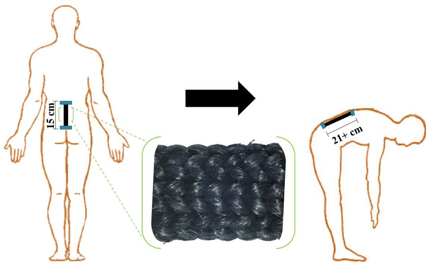
We present an alternative to the current clinician measurement of spinal flexion: the modified Schober's test. By implementing a strain sensor in place of the measuring tape currently used, it is proposed that inter-observer error would be reduced and more consistent measurements would be provided over time.
