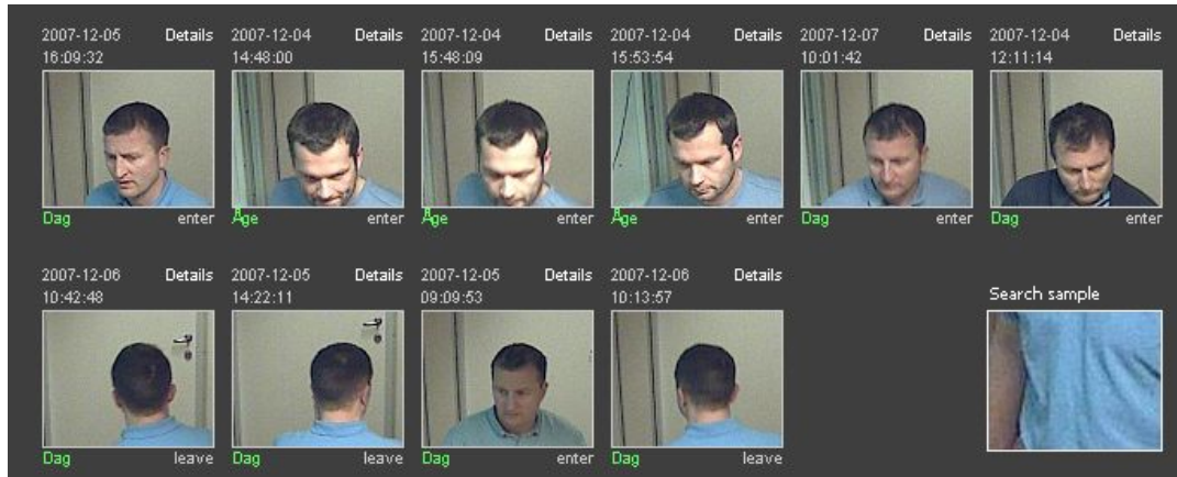
Figure 9. Example search result of persons wearing clothing with similar color to that of a sample input.
