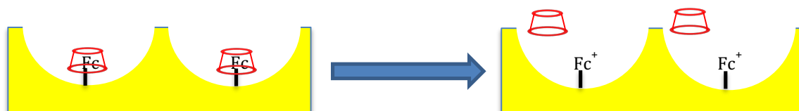
Scheme 4.1 Scheme of the electrochemically controlled release of \beta -CD.
