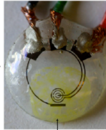
A spread of 30 \mu\text{L} Nafion® on sol-gel membrane
