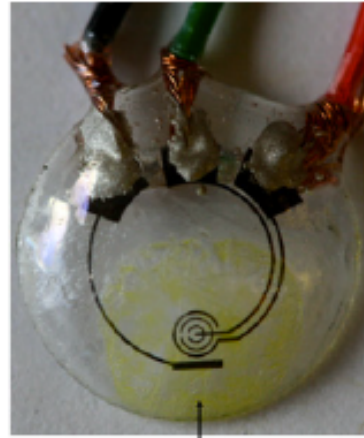
A layer of GOD/titania sol-gel membrane
