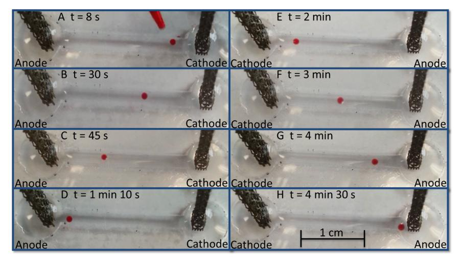
10<sup>-3</sup> M NaCl used as electrolyte, 9 V applied across the solution.
