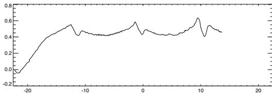
**Figure 5: Ion saturation current versus position across the 'Pastis' system. Conditions of 1.6kW of 60 MHz at 1.2 mBar.**
