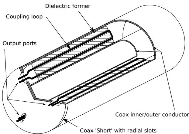
**Figure 3: Schematic of The PSTLD configured to drive 6-tiles. Cut-away showing the coupling loops.**
