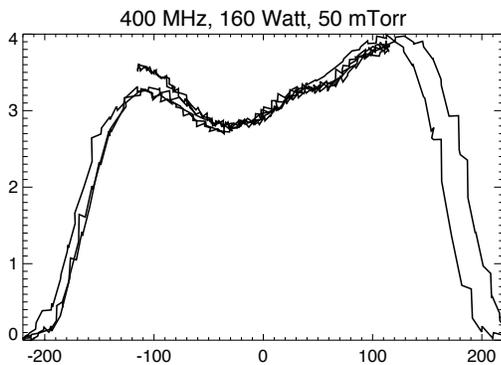
**Figure 6: Ion saturation current across the diameter of the 'Hawaii' plasma source.**
