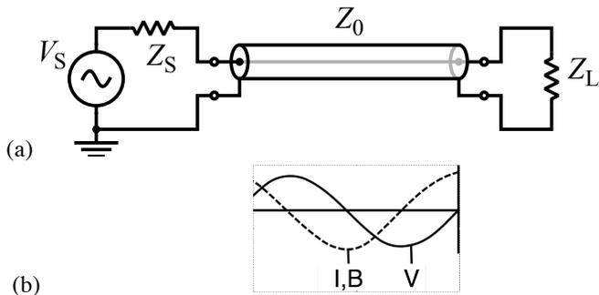
**Figure 2: Transmission line (a) and current and voltage patterns along the length when  $Z_L$  is a short (b).**
