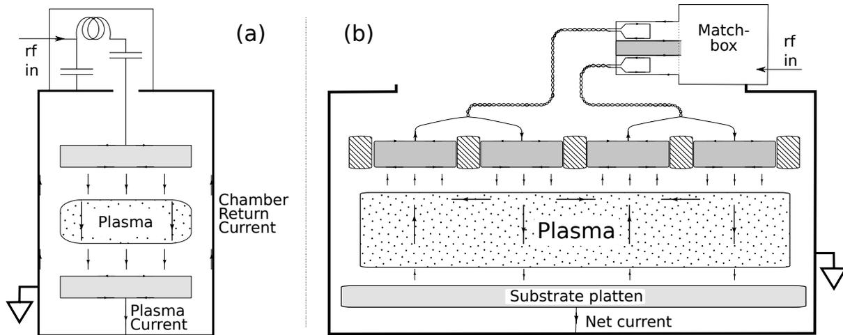
**Figure 1: Traditional CCP plasma system (a) and multi-tile plasma (b). Also shown are the currents at a fixed rf phase.**
