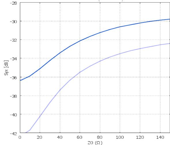
**Figure 4: Cross-coupling between output ports vs port impedance in  $\pm 15$  power splitter configuration (30-tiles). Top curve is adjacent coupling loops, bottom curve is coupling loops diametrically opposed in the coaxial line.**
